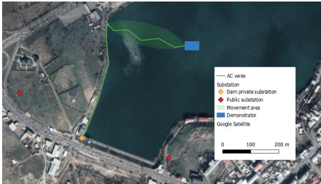
Figure 6: Layout of cables fixed on floats and on the spillway up to the dam substation
