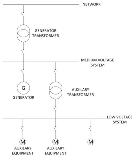
**Figure 6 Basic layout of electrical equipment**
