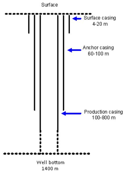
**Figure 2 Casing program for a low temperature well**
