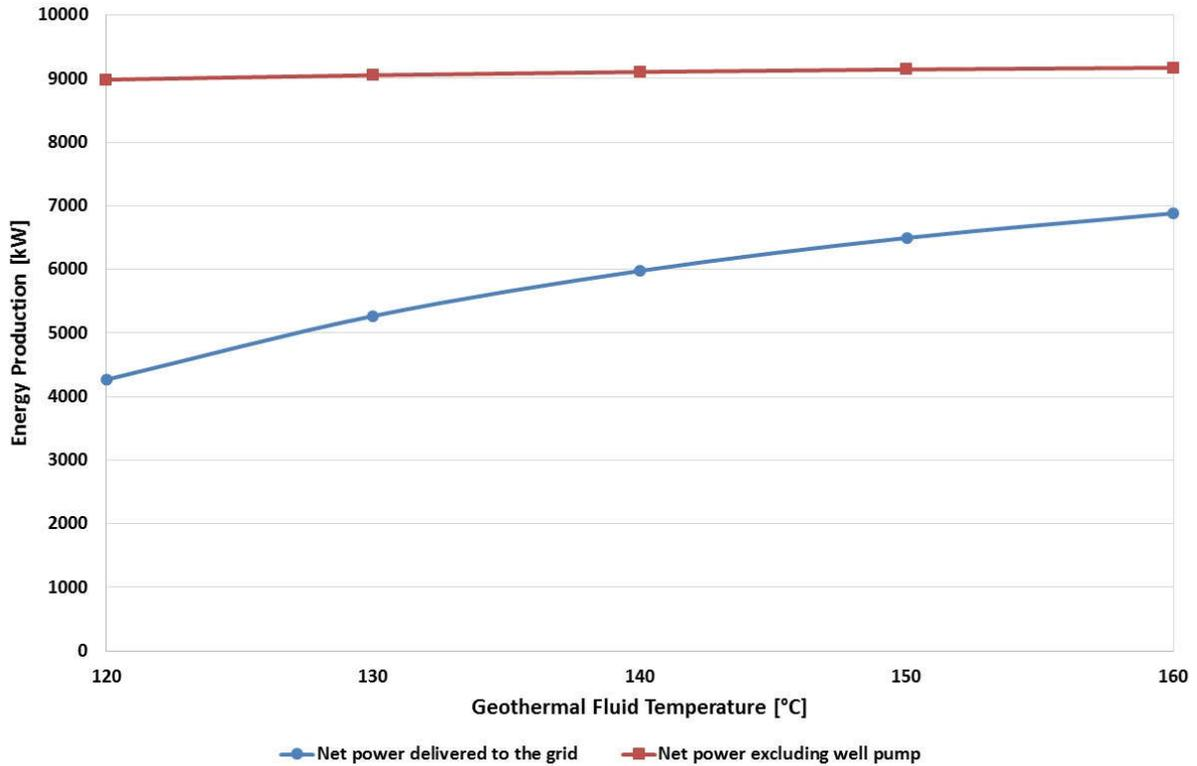
**Figure 8 Net power produced and delivered to the grid as a function of temperature**
