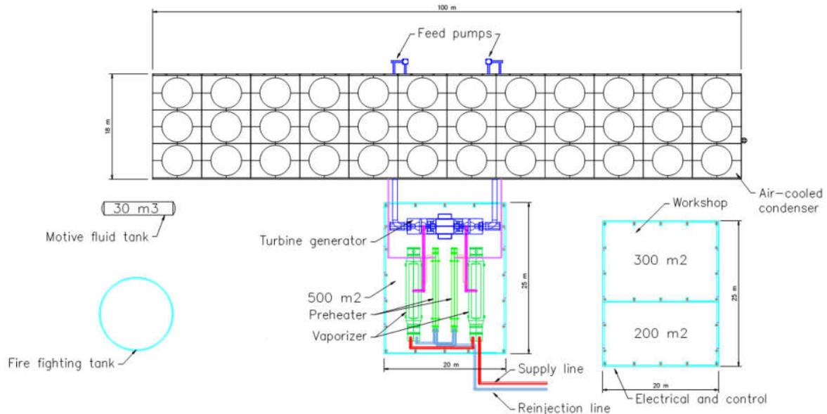
**Figure 5 Simplified setup of a 10 MW power plant with 150°C geothermal fluid temperature as a source.**
