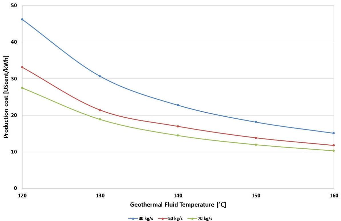
**Figure 11 Production cost of electricity delivered to the grid as a function of geothermal fluid temperature for all cases of geothermal fluid temperature and well flow.**
