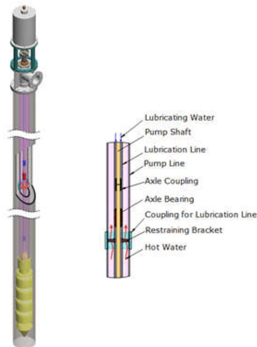
**Figure 3 Line shaft deep well pump**
