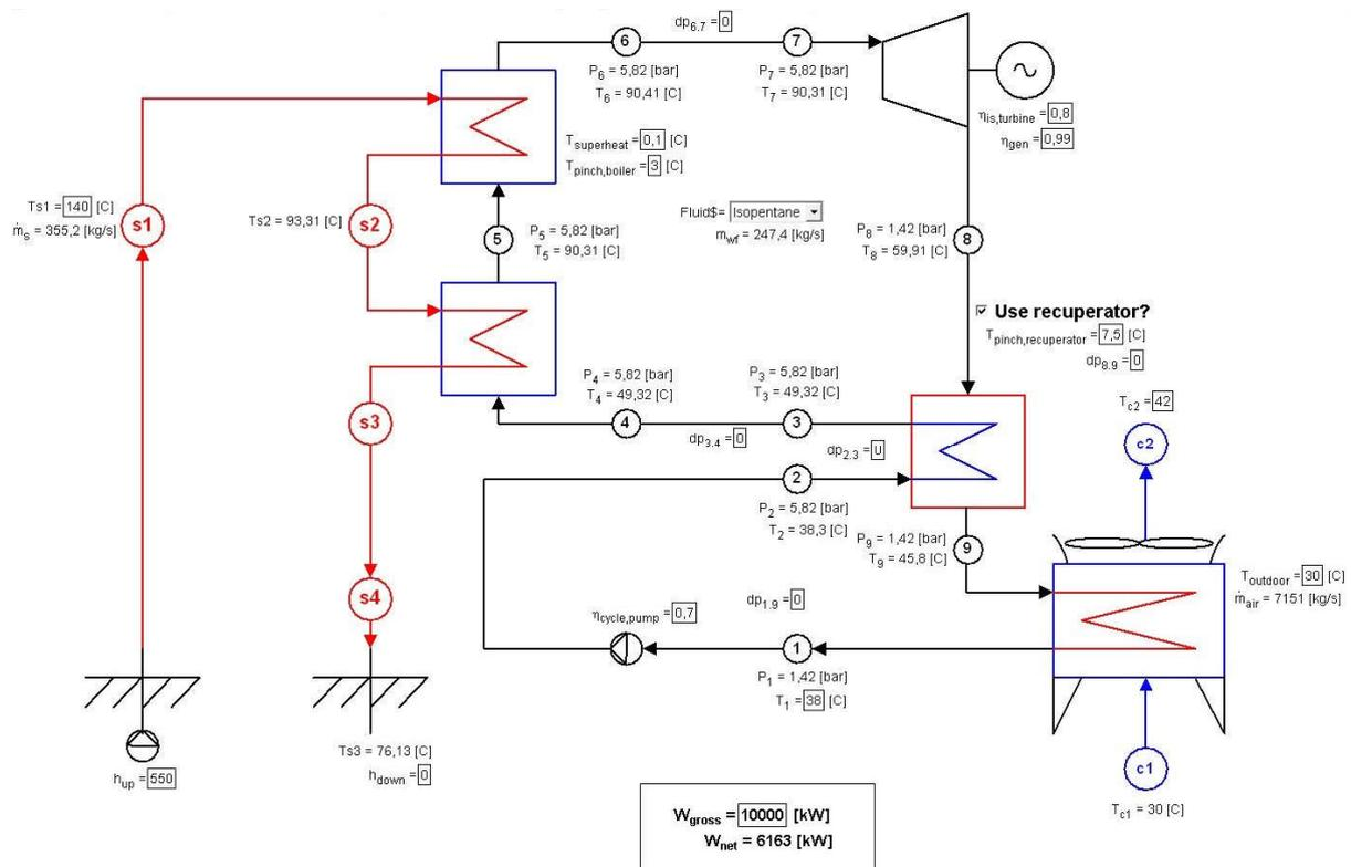
**Figure 7 Heat and mass balance diagram of a 10 MW single stage ORC cycle. Geothermal fluid temperature is 140°C.**
