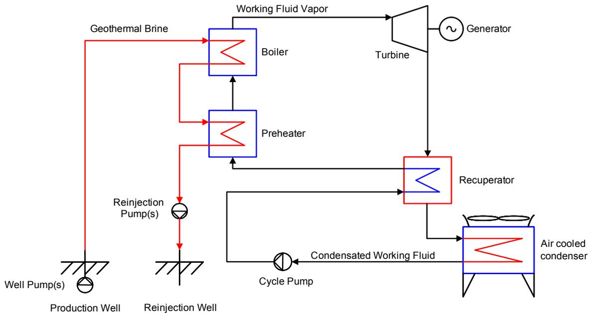
**Figure 4 Binary Power Plant utilizing the Organic Rankine Cycle**
