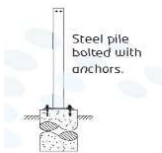
Figure 12 – Krinner screw, reinforced concrete foundation and drive steel profile
