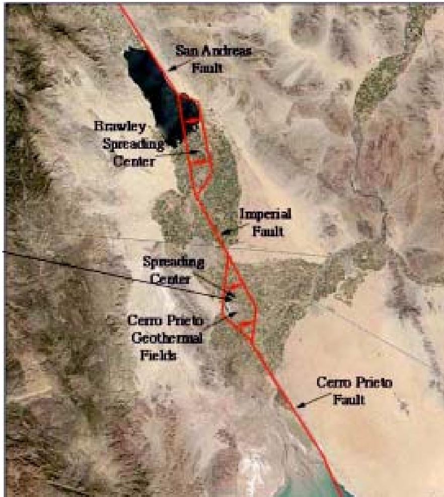
**Fig. 2.55:** A huge hot-water (280-360°C) geothermal system occurs at Cerro Prieto along an offshore segment of East Pacific plates. This field now produces 720 MW of electricity from geothermal reservoirs as deep as 4000 m.
